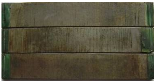
图4 Ni-W-P镀层SSC实验后外观
