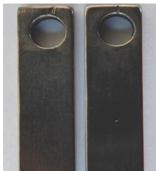
图5 Ni-W-P镀层腐蚀试样外观
