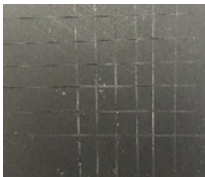
图 6 GO/BTESPT 硅烷复合膜结合力测试结果 Fig.6 Adhesion testing results of GO/BTESPT silane composite film
