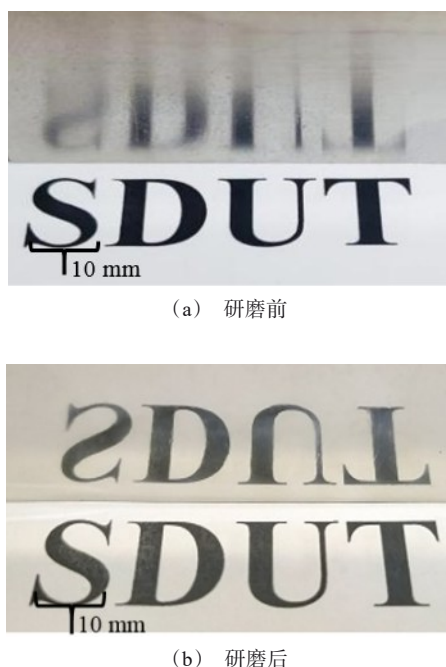
图11 磁力研磨前后310S不锈钢外观
