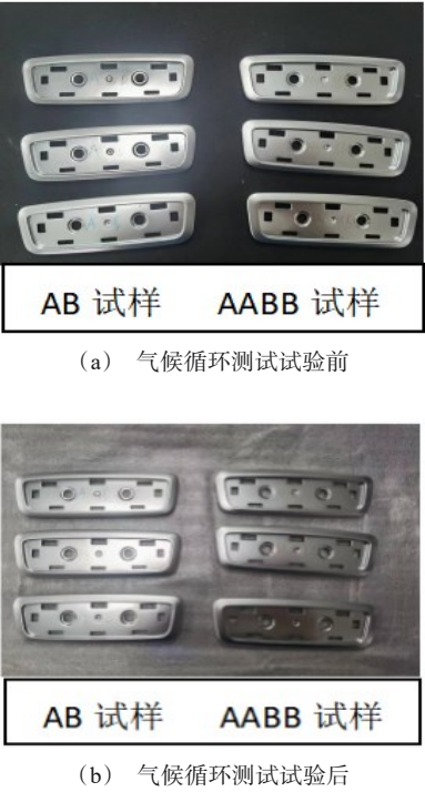
图10 试样AB和AABB在气候循环测试前后的表面状态 Fig.10 Surface state of samples AB and AAB before and after climate cycling test
