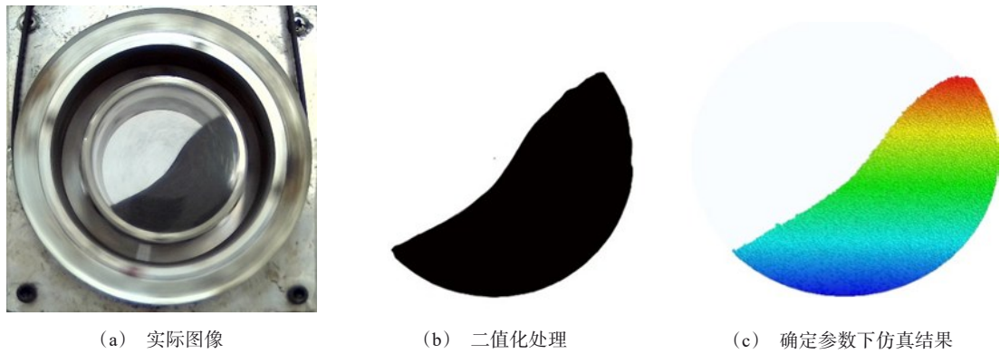
图 3 实际图像与仿真结果对比图 Fig.3 Comparison between actual image and simulation results
