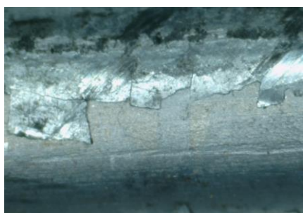
(a) 开裂试样去锌层前
